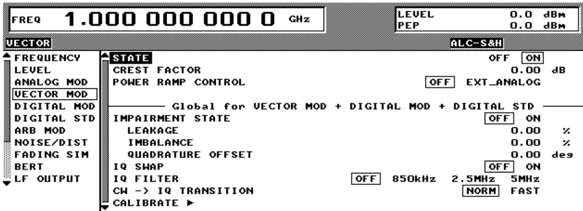
Fig. 2-34 VECTOR MOD menu (preset settings), equipped with option SMIQB47 and IQMOD var. 8 or higher
